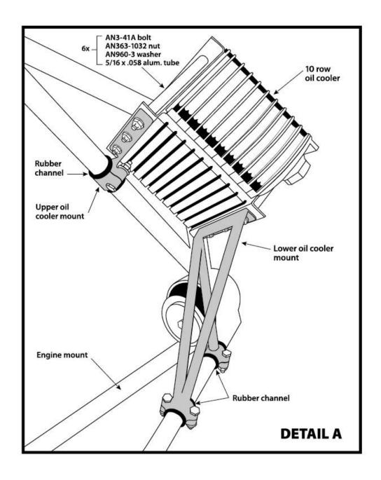
Remove oil cooler leaving the upper and lower mounts in location. Trim the air plenum as needed to sit flat on oil cooler, use the oil cooler to mark then drill the six mounting holes in the plenum, refer to detail B. Fit the cooler/plenum back on the mounts trimming the intake edge of the plenum as necessary to maintain 3/16" clearance from the engine baffle when the oil cooler/air plenum is bolted to the mounts.
