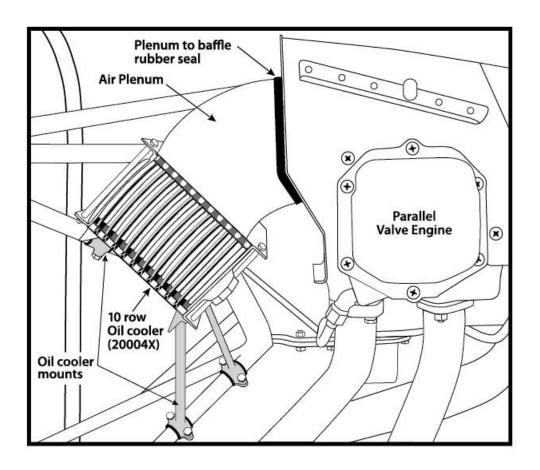
These instructions will guide you through the installation of the oil cooler mount and 20004X or equivalent sized 10 row oil cooler.
